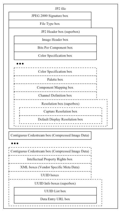
Figure I.1 – Graphical representation of a JP2 file. Dashed lines indicate optional boxes. (Modified from ISO/IEC 15444-1:2004, "Information technology – JPEG 2000 image coding system: Core coding system", figure T.800\_FI.1)
